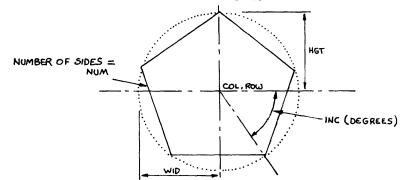
COL and ROW are the centre of the polygon. WID is the horizontal radius and HGT is the vertical radius. INC is the inclination in degrees and NUM is the number of sides. If NUM is large, or less than three, a circle (or ellipse) is drawn instead of a polygon. For example, POLY 0,32,32,32,32,5,0 draws a pentagon in the top left of the screen. POLY 0,32,32,32,32,5,36 draws another one over it, while POLY 0,32,32,32,32,0,0 draws a circle.
