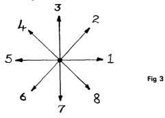
When a value of zero is returned by JSl or JS2, this indicates that the joystick is in its unused position.
